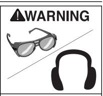
Operating this nailer can propel objects into the air, causing immediate eye damage. To protect yourself, always wear American National Standards Institute (ANSI) approved safety glasses or goggles when operating this equipment. In addition, this nailer discharges at 85-90 decibels. To protect your hearing, always wear ANSI approved ear protection when operating this nailer.
